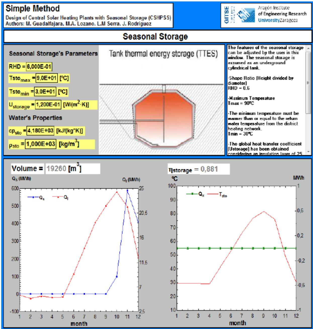
Fig. 3: Seasonal Storage window of the developed software for the analysis and evaluation of CSHPSS.
