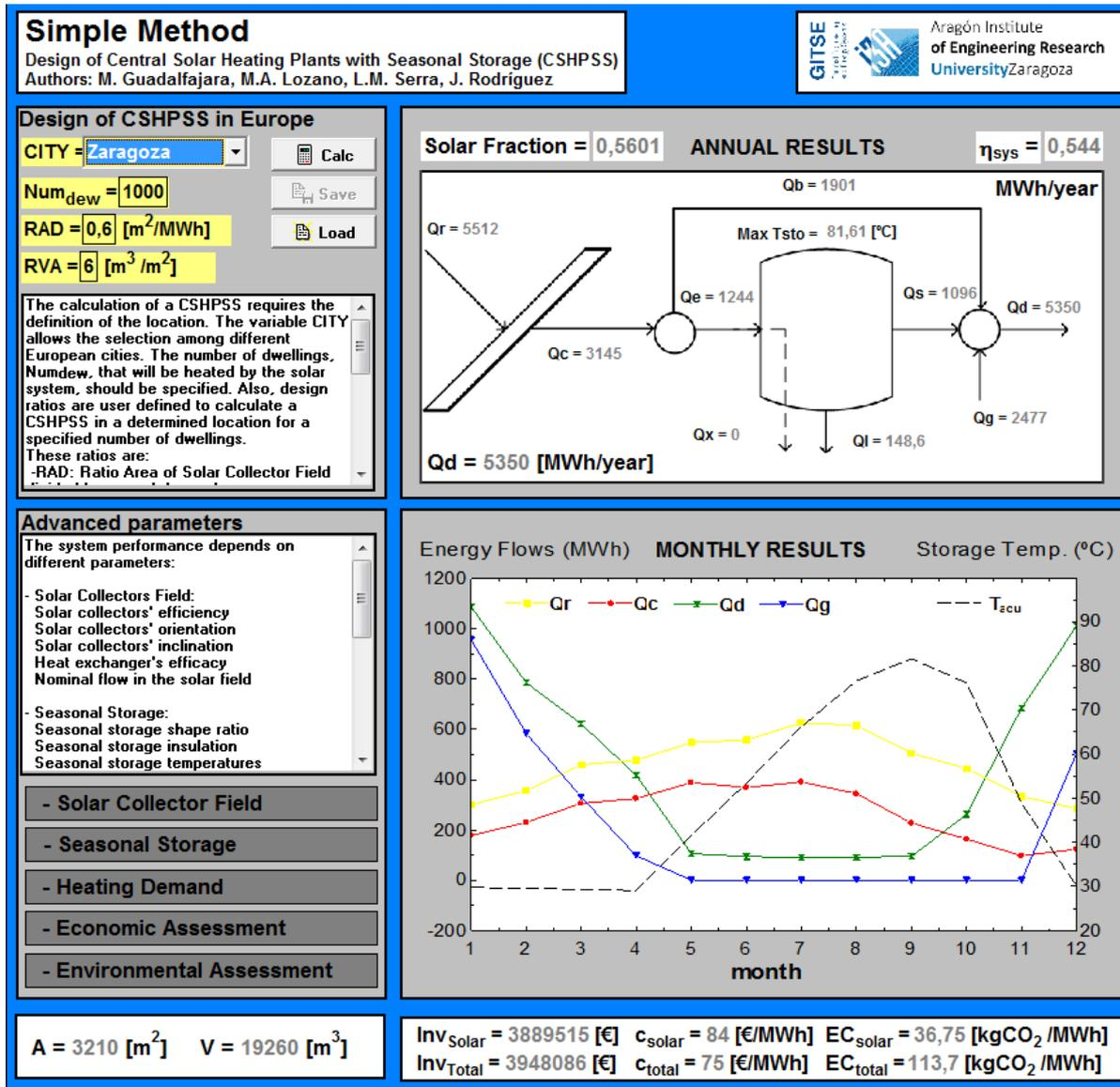
Fig. 1: Main window of the developed software for the analysis and evaluation of CSHPSS.
