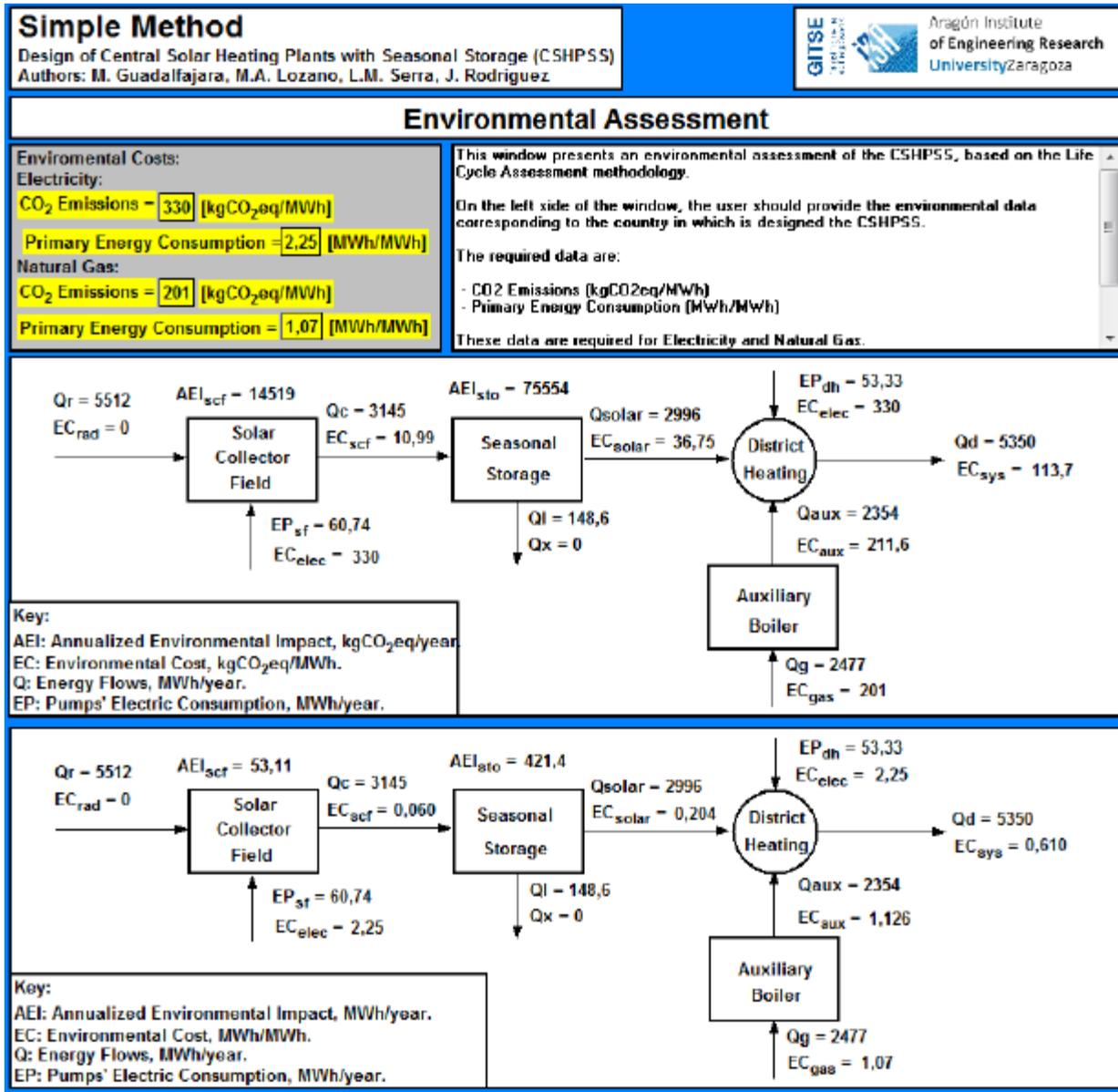
Fig. 6: Environmental assessment window of the developed software for the analysis and evaluation of CSHPSS.
