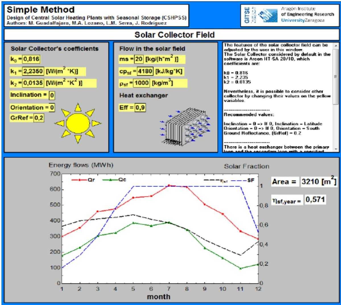
Fig. 2: Solar Collector field window of the developed software for the analysis and evaluation of CSHPSS.
