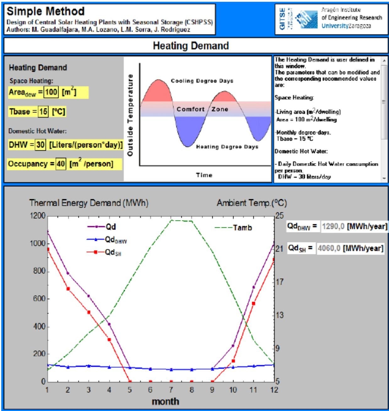
Fig. 4: Heating Demand window of the developed software for the analysis and evaluation of CSHPSS.
