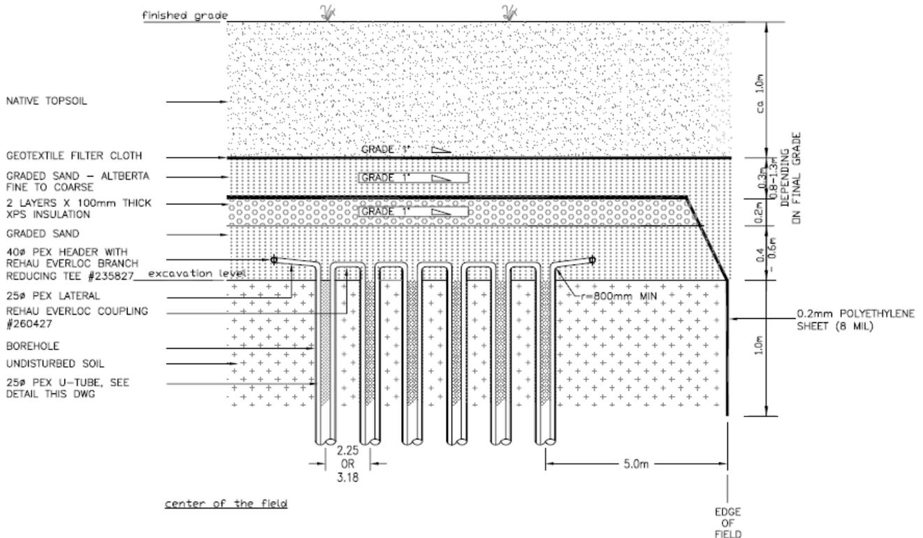
Figure 2. Cross-section of the top portion of one BTES circuit
