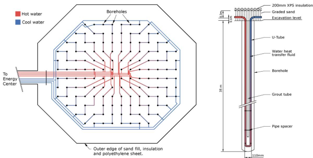
Figure 1. Layout of a borehole thermal energy storage and cross-section of a single borehole and u-tube
