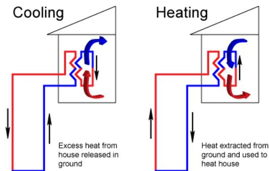
Figure 20: Heating and Cooling with Geothermal Energy
