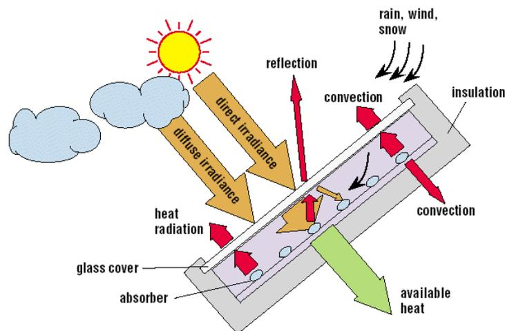
Figure 7: Flat Plate Collector<sup>15</sup>
