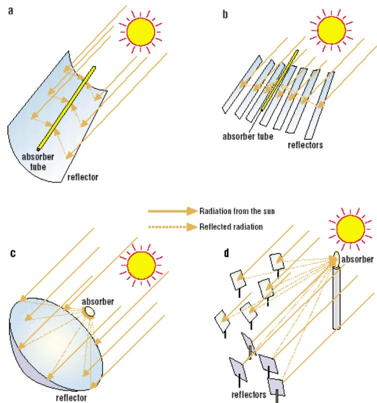
Figure 8: Concentrating Collector Types<sup>16</sup>
