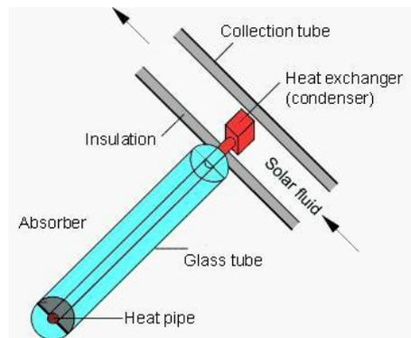
**Figure 9: Evacuated Tube Collector<sup>17</sup>**
