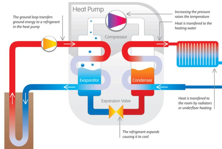
**Figure 16: Heat Pump Cycle**<sup>31</sup>
