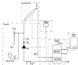
Figure 11: Schematic Collector Cycle
