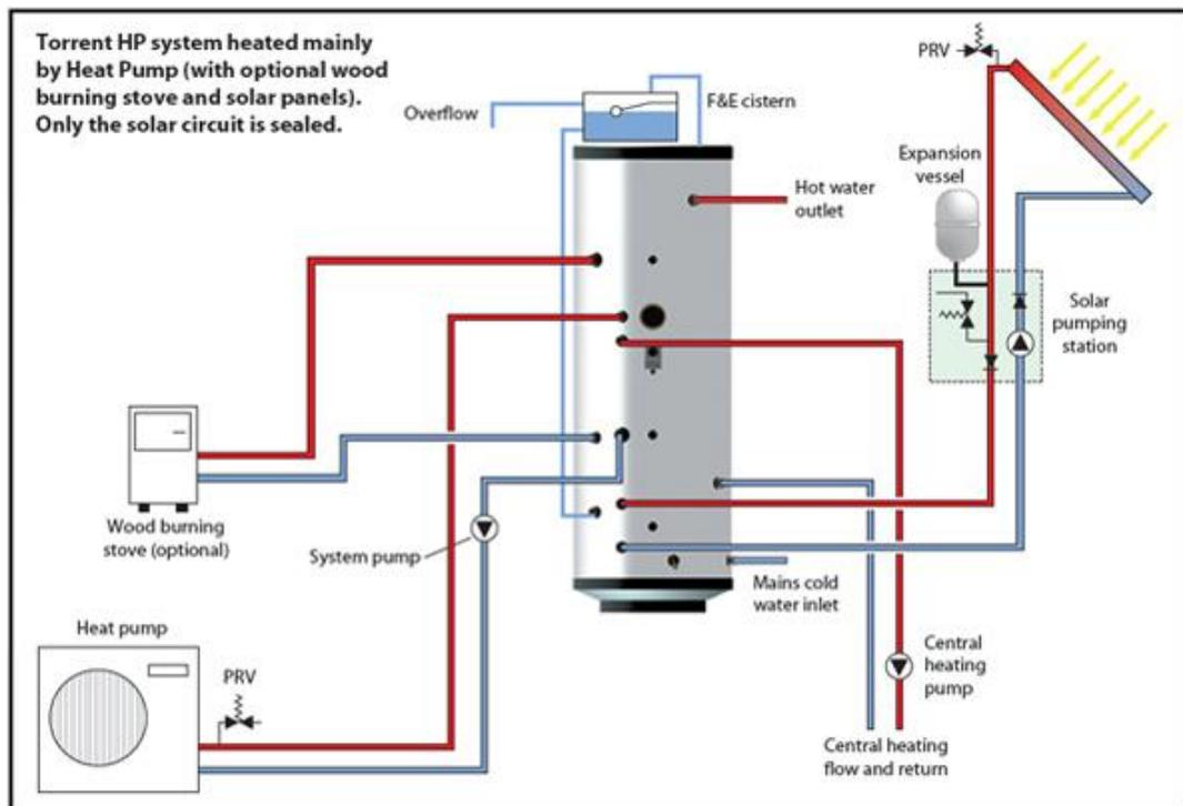
Figure 13: Solar Combination Systems<sup>21</sup>
