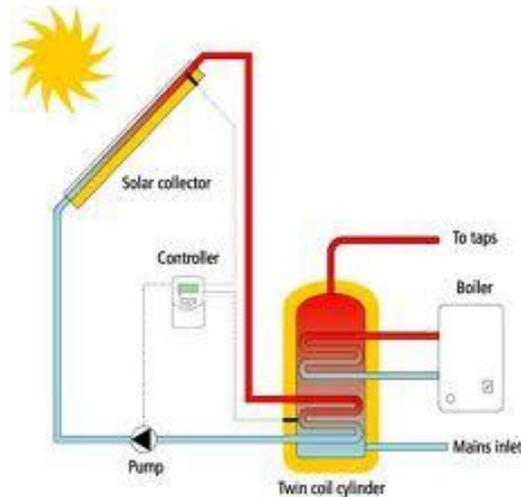
Figure 2: Basic working principle<sup>5</sup>
