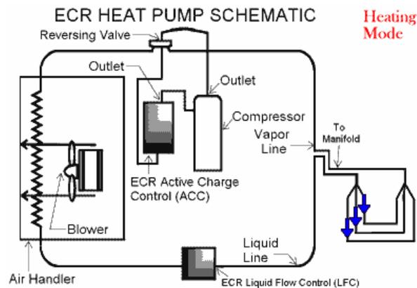
Figure 19: Schematic Heat Pump<sup>45</sup>
