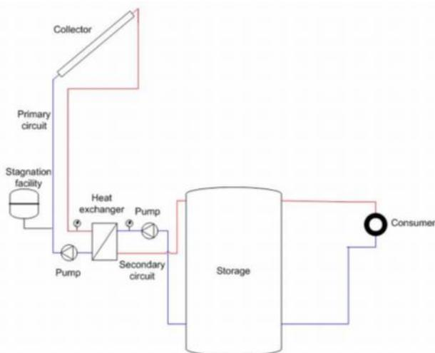
Fig. 1: Basic scheme of a solar thermal plant
