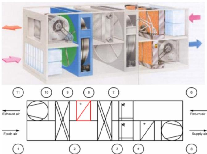
Fig. 8: Schematic of an Desiccant cooling system
