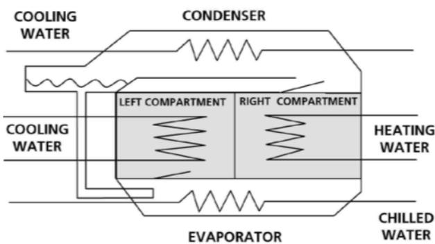
Fig. 6: Schematic of the internal chambers of an adsorption chiller [Error! Bookmark not defined.]
