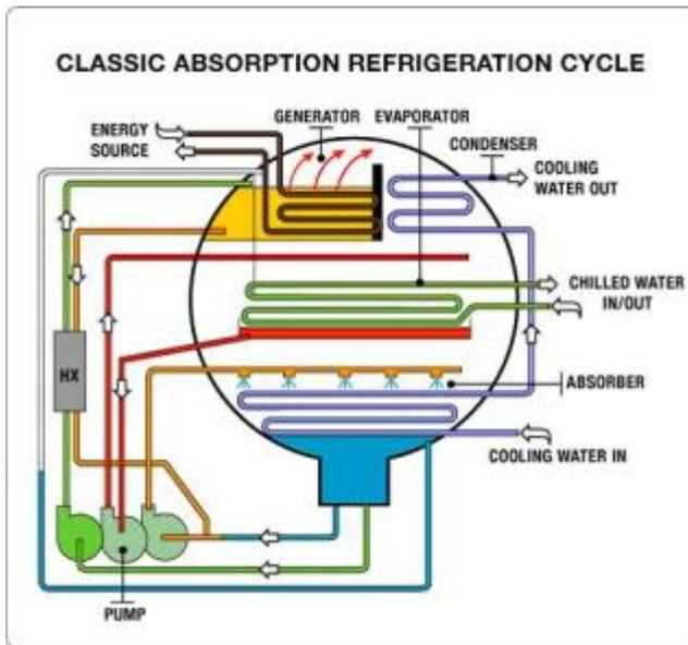
Fig. 4: Schematic of an absorption chiller [2]
