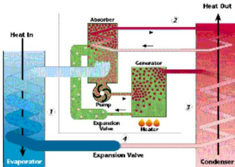
Fig. 16: Absorption heat pump
