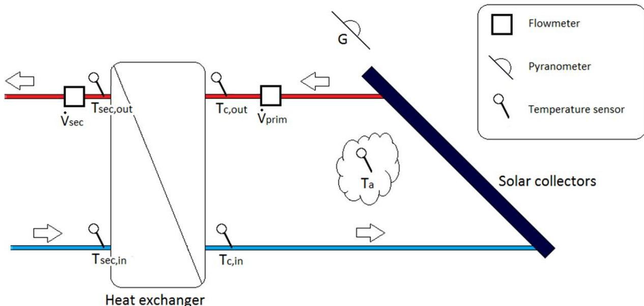
Figure 1. Schematic drawing showing the measurement points. (Source: PlanEnergi)
